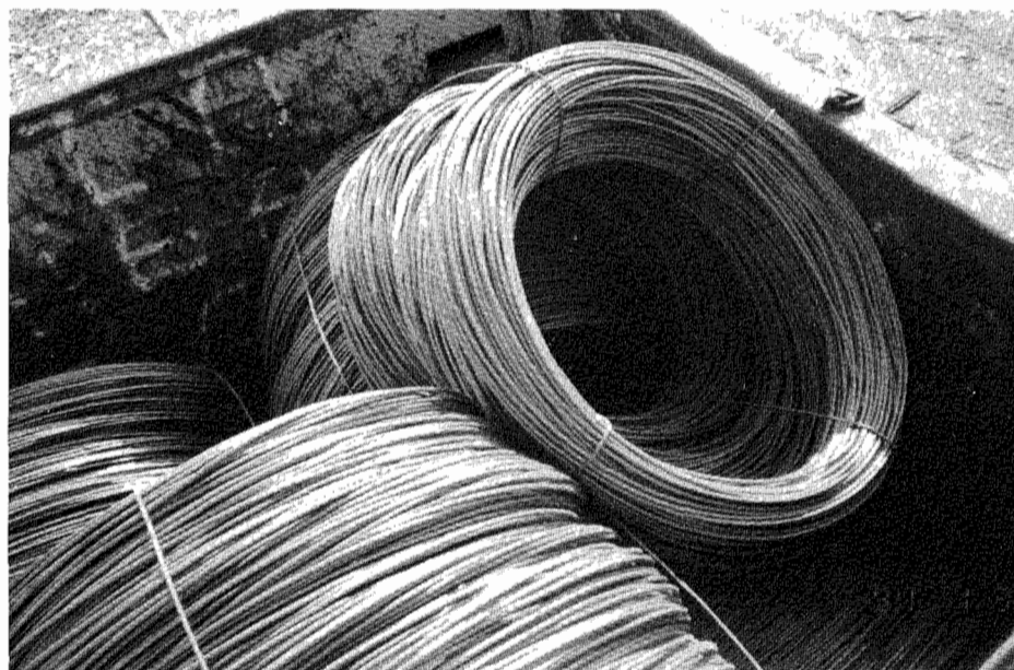
The 12-Inch Mill Team No. 2 found the problem of coils becoming loosened during shipment to be very serious. Many coils shipped by rail ended up in the condition shown in the photo above. The team's solution was to secure the coils with a wider steel band, fastened with a clip (below).
