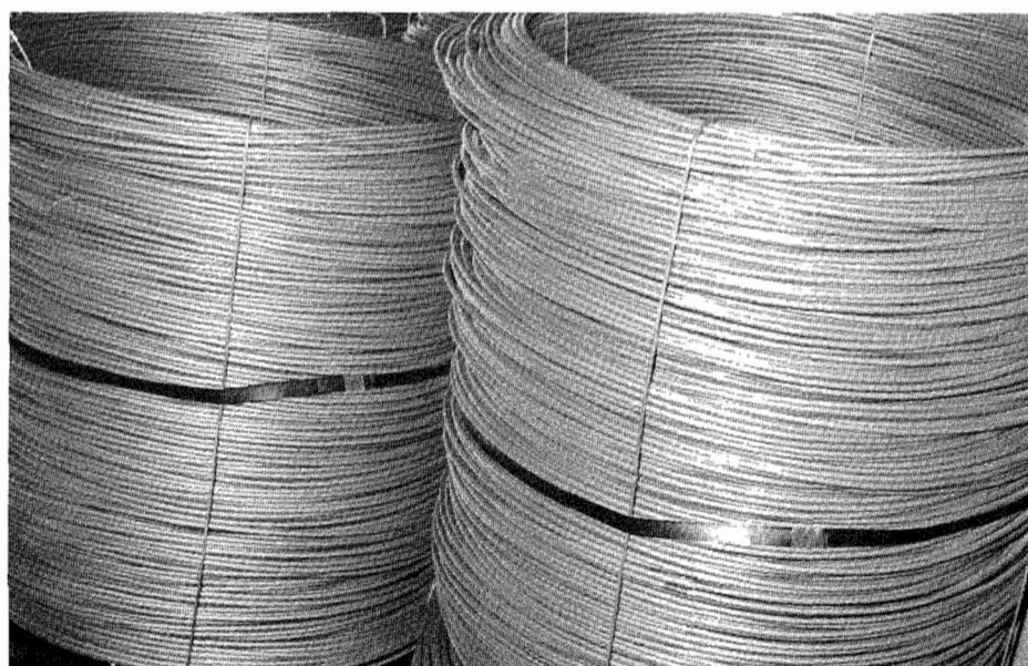
The 12-Inch Mill Team No. 2 found the problem of coils becoming loosened during shipment to be very serious. Many coils shipped by rail ended up in the condition shown in the photo above. The team's solution was to secure the coils with a wider steel band, fastened with a clip (below).
