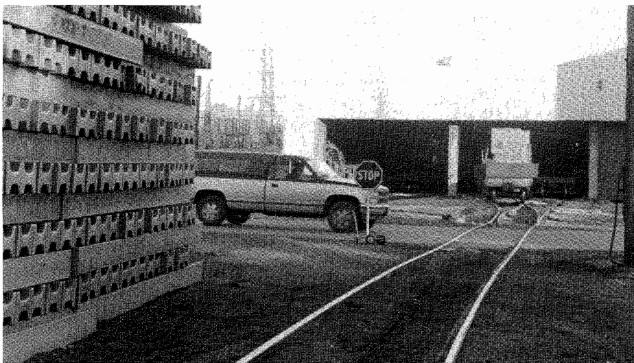
The beam blanks pictured above on the left block the view of the switchman. Because of the blanks, he can't see the truck until the truck is right at the track.
