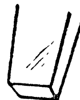
Cut masonry nails have a square "cut" point.
