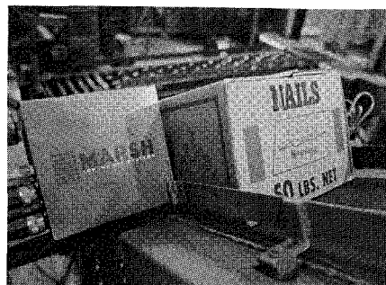
The Marsh ink jet system sprays production information on two sides of each box.
