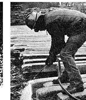
Kenneth Kennedy, Scarfer Helper, is shown identifying the semi-finished slabs just before they are scarfed in the left photo. Center, Keith Kendall is one of the Scarfers at the yard who clean up the imperfections in the slabs before they are taken to the 20-24 Inch Mills. At the right, Scarfer Ted Hardt is shown "cupping" the semi-finished slab so it passes through the rollers of a roughing mill more easily.
